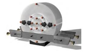
**Standard CT Dose Phantoms**, Model 007 & 007A. Both fully comply with the FDA performance standard, 21CRF1020.33. Model 007A features a pediatric inserts as well as the adult head and body.
