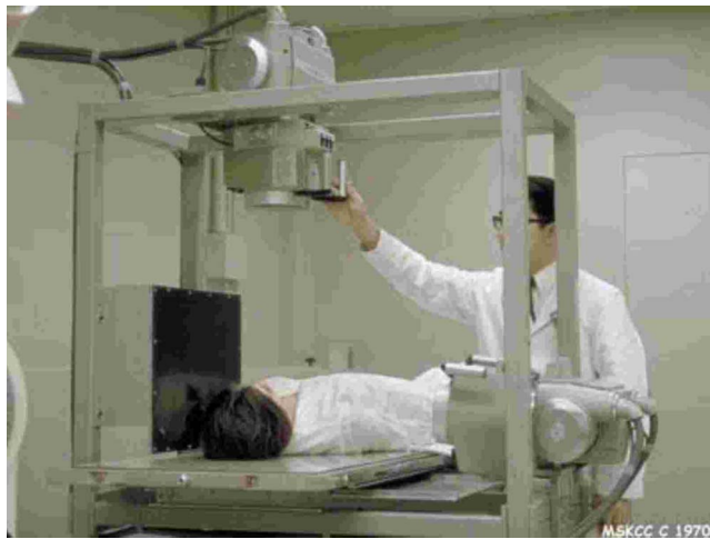
FIG. 17. Apparatus for the automatic localization of implanted seeds c 1970 (MSKCC).
