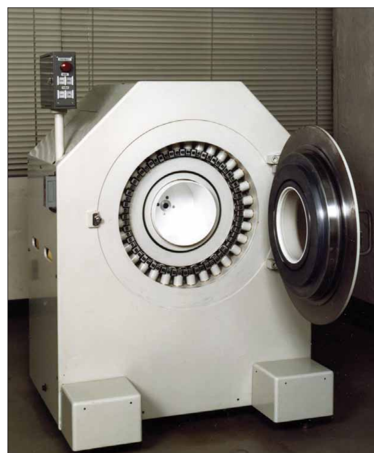
Figure 2 The first PET scanner, Positologica-I, in Japan (1979).
