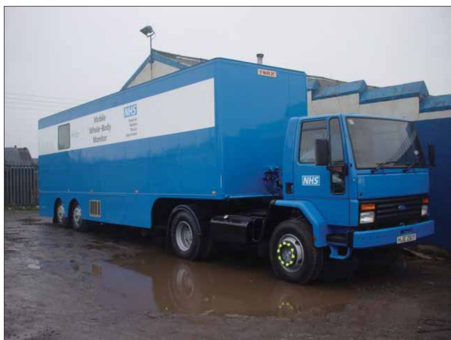
The mobile whole body counter used to measure uptake of radioactivity in the population of UK following the Chernobyl accident. Professor Boddy led the project.
